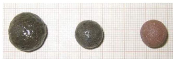
Figure 1: Lightweight aggregate prototypes. Protótipos de agregado leve.
