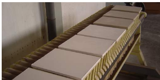
Figure 1: View of extruded ceramic pieces. Vista de pavimento extrudido.
