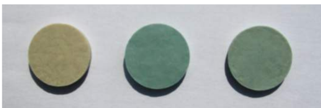
Figure 1: Application tests (10 wt%) of the T1-Ni (center) and sludge-based (right) pigments on stoneware paste (on the left). Testes de aplicação (10 wt%) de T1-Ni (centro) e pigmentos à base de lamas (direita) em pasta de grés (esquerda).
