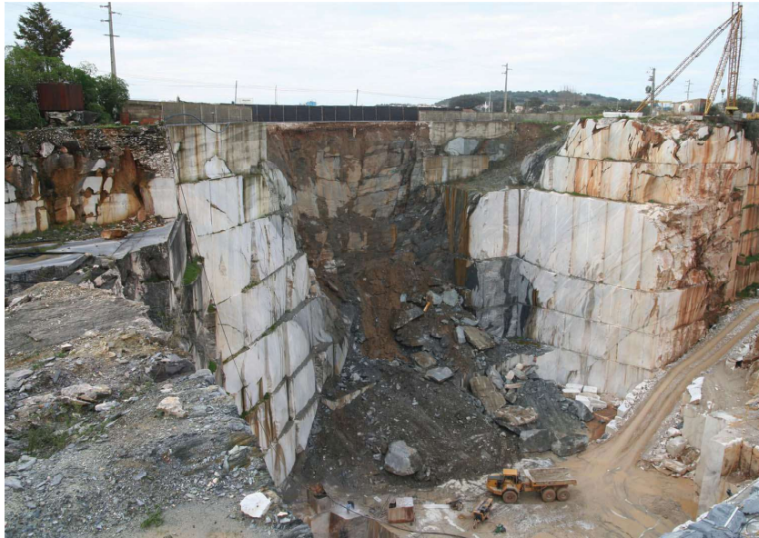
Figure 2. Rock fall of the southwest slope of the quarry induced mainly by the effect of the water pressure within the discontinuities. This accident has also cut a road which profile is visible on the top of the slope. This quarry is located at point 2 in Figure 1.
