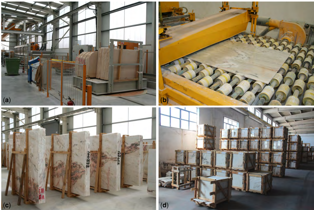
Fig. 6. Images of marble processing plants near Vila Viçosa. (a) Partial view of a polishing slab line. (b) Details of polished slab at the end of the line. (c) Slabs ready to export. (d) Tiles with several dimensions and marble varieties packed to export overseas. Photos were taken in the following companies: Plácido José Simões S.A.; Criamármore – Mármore de Portugal Lda.; ETMA – Empresa Transformadora de Mármore do Alentejo, S.A. and Empresa Marbrito, Indústrias Reunidas de Mármore, Lda.
