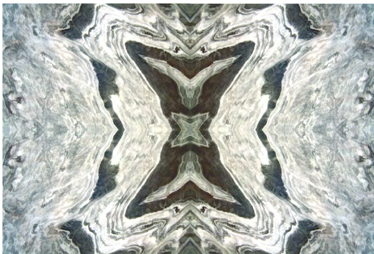
Fig. 4. This picture shows an example of geometric patterns obtained by polishing the Ruivina (dark blue to grey colour marble variety) marble slabs in open book.
