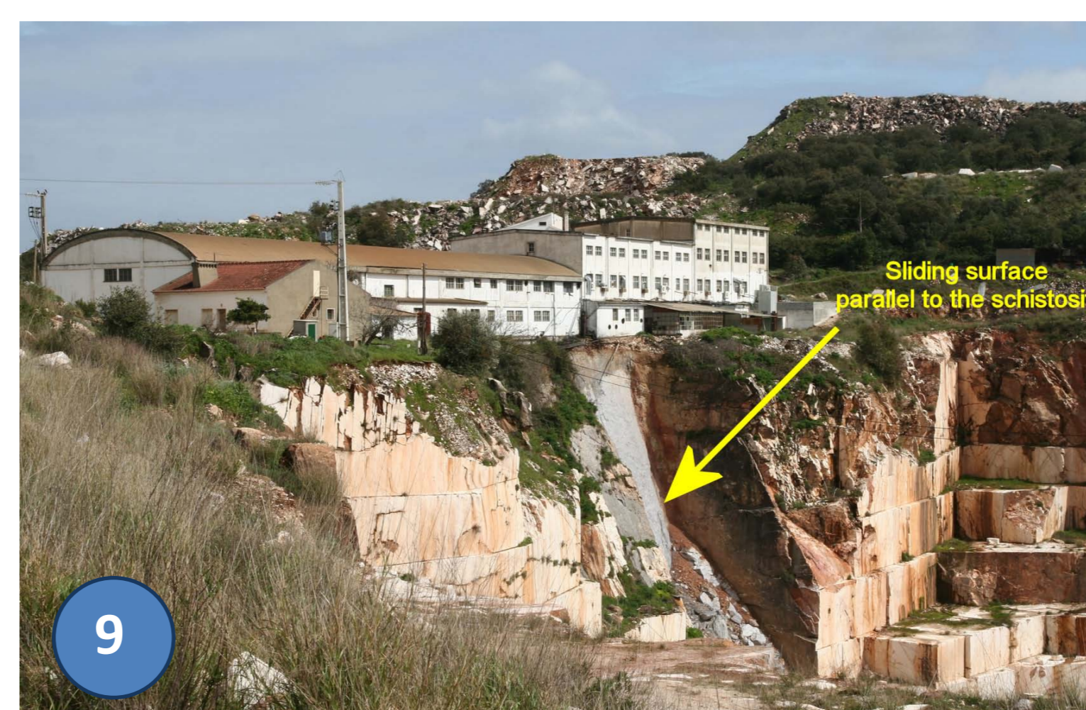
Figure 8. Example of procedure not appropriate of marble quarrying that can decrease the safety of people and cause material damage.
