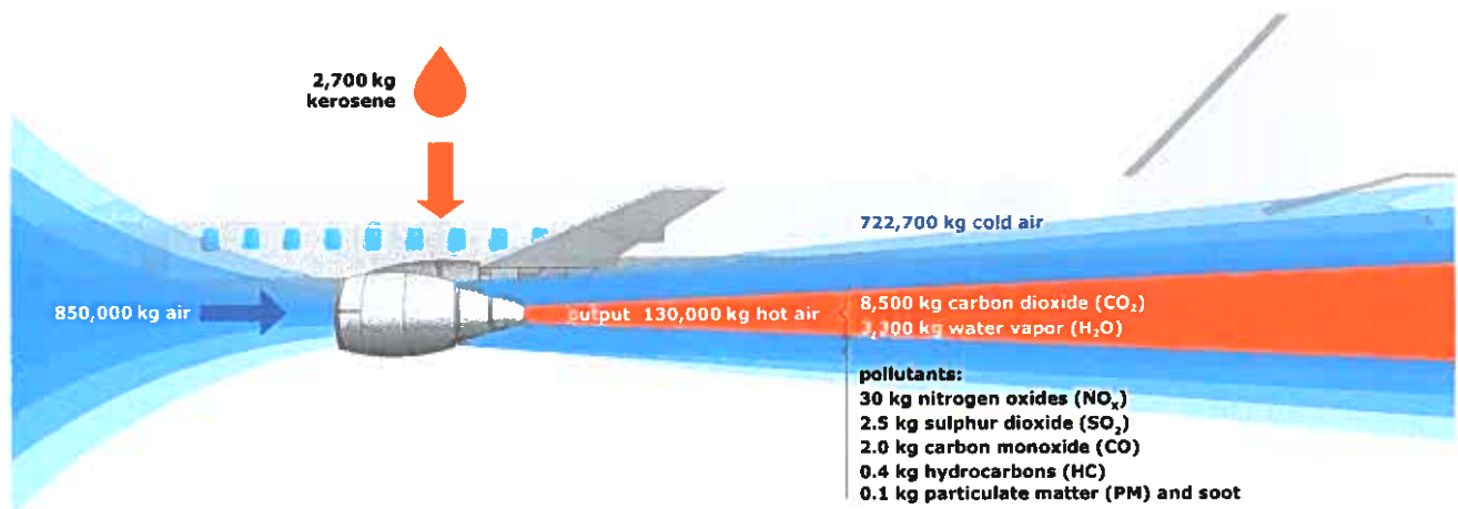
Figure 1.8 Emissions from a typical two-engine jet aircraft during 1-hour flight with 150 passengers (Source: FOCA)
