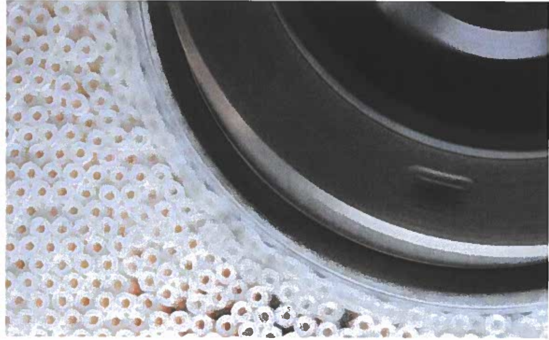
Above: Filtered tobacco units hollow acetate tubes.
